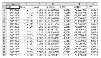
The file has the following format: the first line is a header where all the sensor names are displayed (two times each – e.g. "a (W), a (dBm)"), each next line represents a measurement of all active sensors. The results are saved both in Watt and in dBm, together with the date and time when they were recorded. No power values for sensors in scope or time slot modes are saved (e.g. sensor "i" on the picture).
